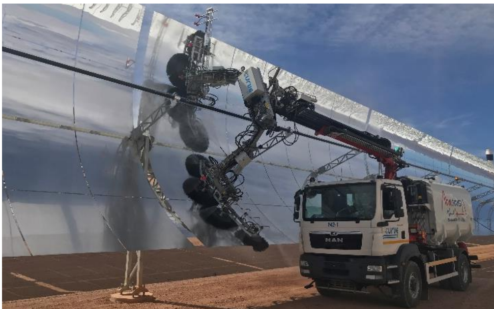
Picture 2: CURVE B Brushes - Details @ Noor 2 CSP plant (Copyright: ECILIMP Termosolar SL (Spain))
