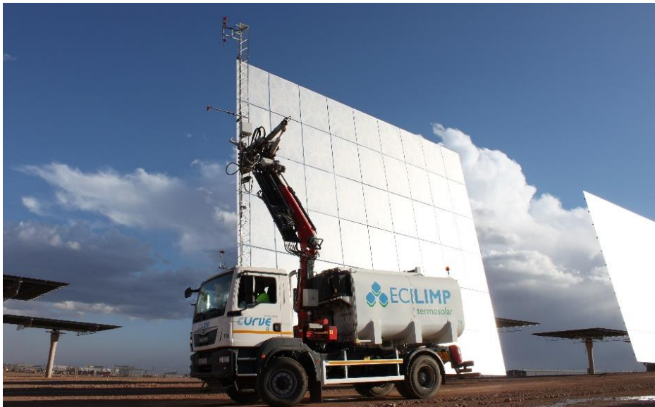
Picture 1: CURVE B truck using HELIOS Cleaning Tools @Noor3 CSP plant (Copyright: ECILIMP Termosolar SL (Spain))
